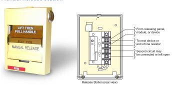
The manual release station is a normally-open, dry contact signal initiating device. The 276A-REL is a single-action station that requires the user to pull the release handle to initiate the release of a fire suppression agent. The 278A-REL (shown) is a double-action station that requires the user to raise the upper door, then pull the release handle to initiate the release.
